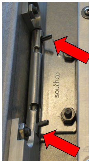
Figure 5-8) Door Hinge Locked
