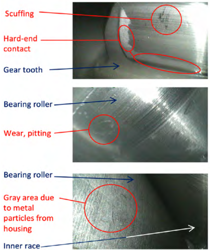
Figure 6. Endoscope camera pictures of the parallel gears and bearings: IMS gear (top), IMS-NRE bearing (middle), IMS rotor side bearing (bottom).
