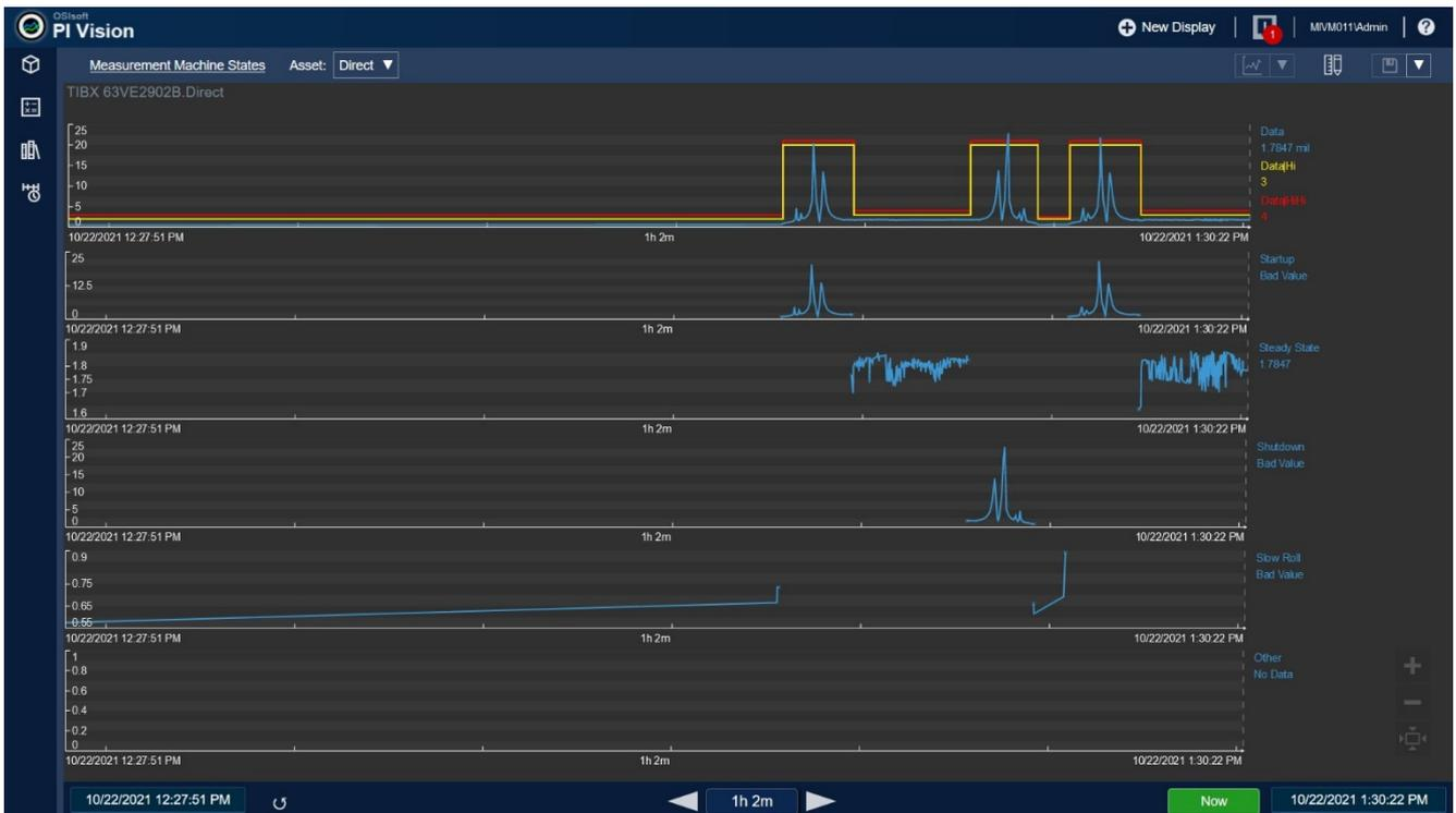
Figure 1: Screen plot shows five machine states based on speed for a steam turbine starting up twice and being shut down once. The alarm limits for the run up and coast down machine states are shown in the upper plot. The alarm limits are not shown for the running or turning machine states but these too will have individual alarm limits. A fifth machine state shown below has no data yet.
