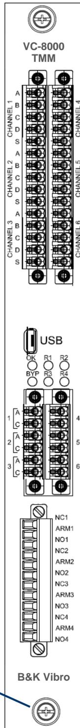
Captive thumbscrew for securing TMM in SETPOINT rack slot.
