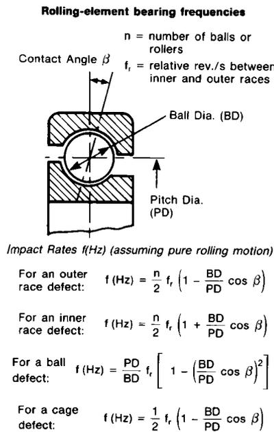
Fig. 1. Formulas for calculating bearing frequencies
