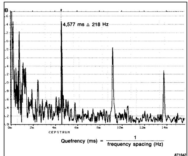
Fig. 6. The family of harmonics in Fig. 5 shows up in the cepstrum as a distinct peak whose quefrency corresponds to the frequency spacing of the harmonics. A number of harmonics (equivalent to harmonics in a normal spectrum) are also present.
