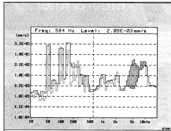
Fig. 2. CPB spectrum comparison of the vibration of a 110 kW motor. The dark line is the "good-condition", reference mask against the current spectrum (light line) is compared.
