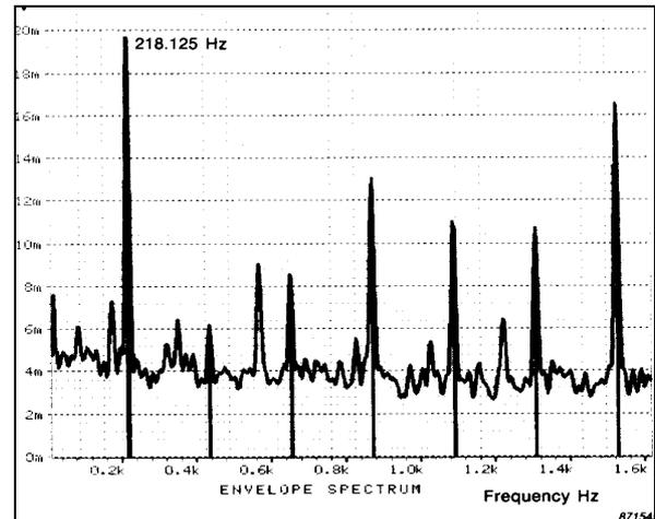
Fig. 7. The envelope spectrum corresponding to Figs. 5 and 6, showing a harmonic series of the BPFO (Outer race defect)
