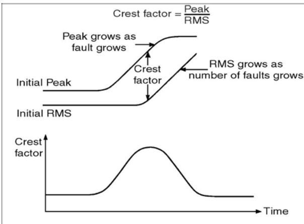
Fig. 3. The Crest Factor principle
