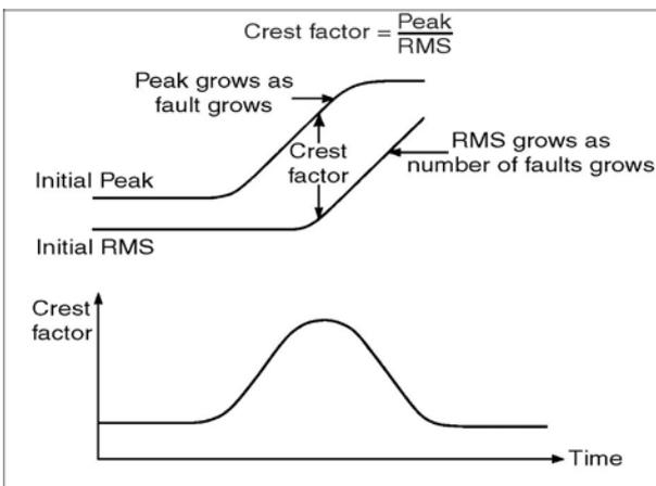
Fig. 3. The Crest Factor principle
