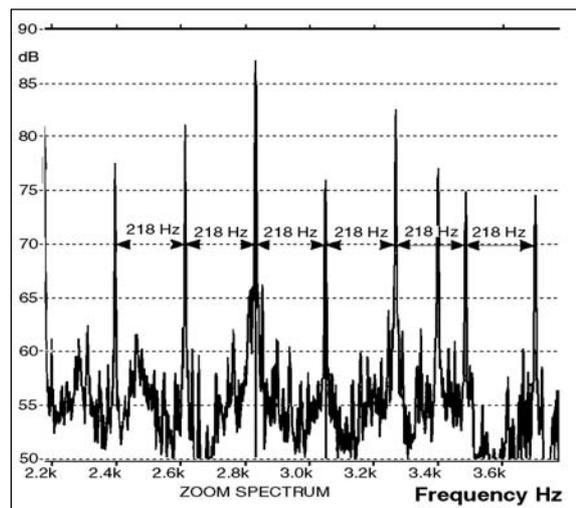
Fig. 5. Zoom spectrum showing harmonics corresponding to the ball-pass frequency outer race (BPFO). When the bearing was stripped down, eight months after the fault was first detected, a spall was discovered on the outer race.
