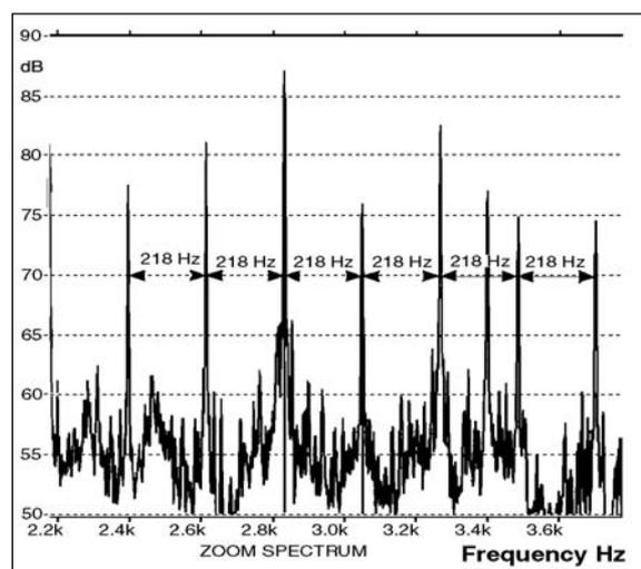
Fig. 5. Zoom spectrum showing harmonics corresponding to the ball-pass frequency outer race (BPFO). When the bearing was stripped down, eight months after the fault was first detected, a spall was discovered on the outer race.
