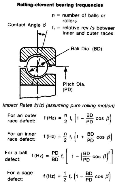
Fig. 1. Formulas for calculating bearing frequencies
