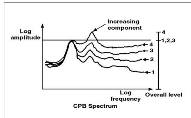
Fig. 4. A CPB spectrum comparison gives earlier warnings than monitoring of overall vibration - the level of overall vibration only increases after an increasing component has become the highest peak in the spectrum
