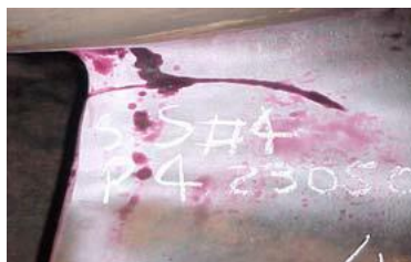
Figure 6. Left picture: One of the two cracks caused by vortex pressure pulsations during a relatively short time. Right: Lowpass plot showing the increased vortex pressure pulsation levels at day 8.
