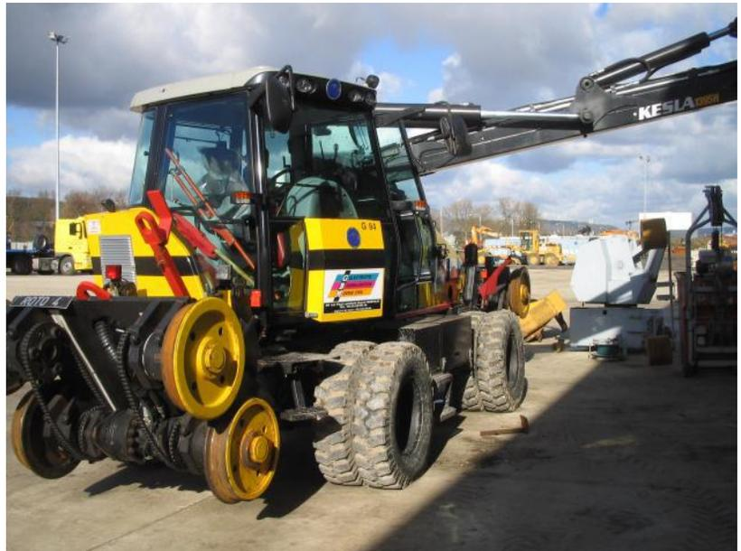
Figure 1. The railroad version of the land clearing tractor .
