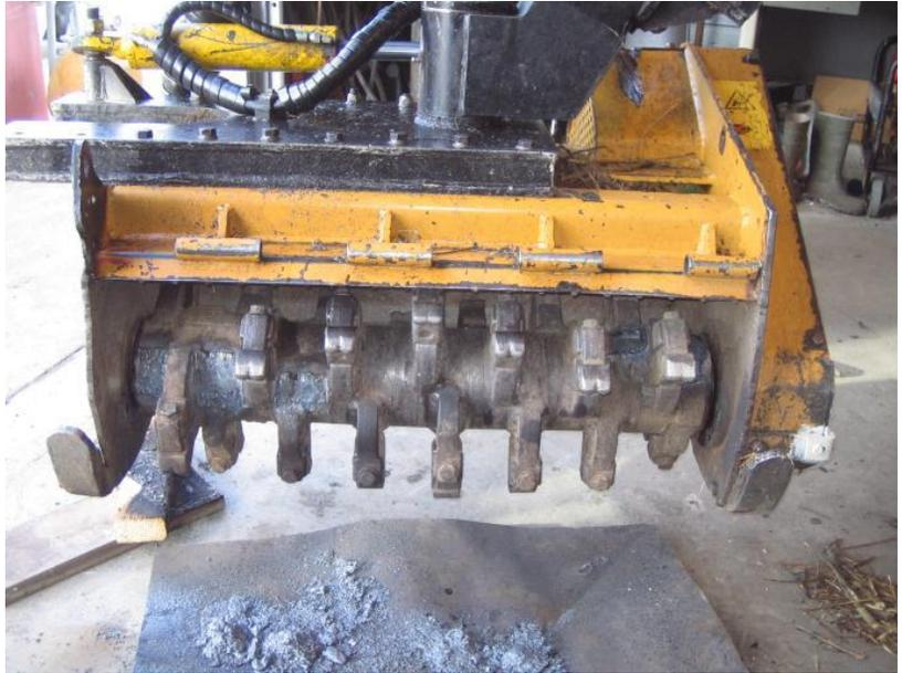
*Figure 2. Close-up of the rotary mulcher head of the land clearing tractor, showing the rotor that has to be balanced.*
