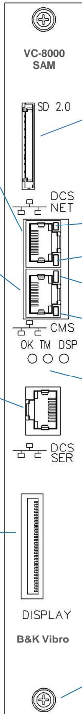
Captive thumbscrew for securing SAM in SETPOINT rack slot.
