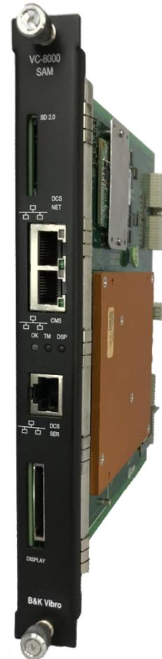
The SAM is not in the critical machinery protection path; therefore, its inclusion enhances basic rack functionality without affecting machinery protection, even in the unlikely event of a SAM failure. The SAM resides in rack slot #2 and uses 24 V<sub>DC</sub> instrument power as supplied by the SETPOINT Rack Connection Module (RCM). An additional SAM can be installed in rack slot #3 when Modbus redundancy is required.
