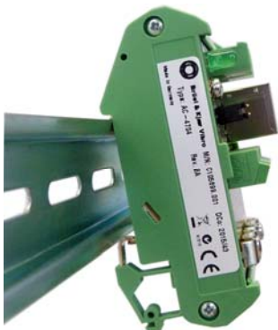
Figure 1) Mounting the top hat rail
