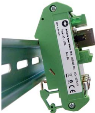
Figure 2) Mounting the top hat rail
