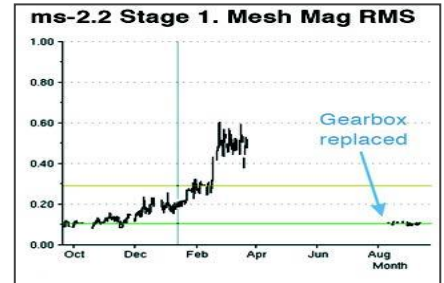
Figure 1: The trend plot showing the gear mesh frequency trend before and after servicing the gearbox.
