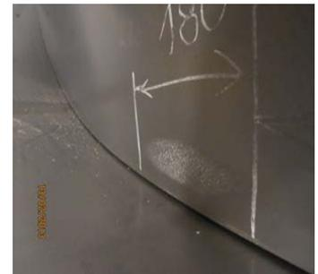
*Figure 1. Runner cavitation before the minimum partial load limit was redefined.*
