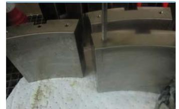
Figure 1. Tilt pad bearings.
