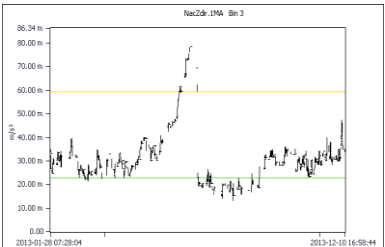
Figure 1. Vibration trend at rotor speed in the downwind direction under increasing pitch misalignment.
