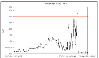
Figure 2. – Low frequency bandpass vibration trend in the downwind direction indicating loose springs in the yaw bearing assembly.
