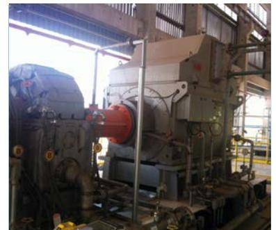
Figure 2. Charge gas compressor
