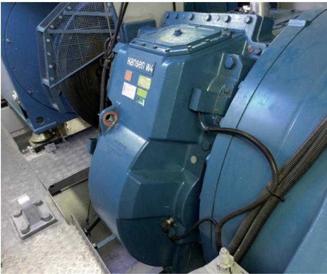
Top: One of the accelerometers used for monitoring the main bearing of the wind turbine drive train. Bottom: Gearbox of the wind turbine drive train. Right: Rattlesnake Road wind farm in Oregon, USA.
