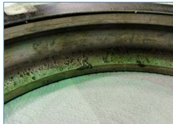
Figure 1. No matter what the cause, it is not always possible to immediately stop the machine when faults are detected. Damaged bearings are often run just before failure, as shown above.
