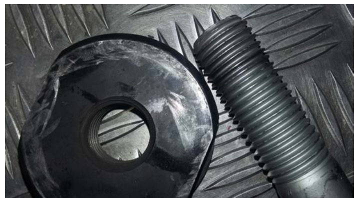
Figure 6: One of the bolts between the disc brake calipers was found lying on the floor plate
