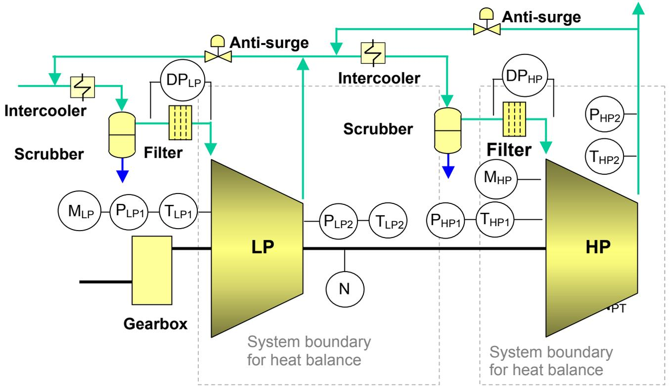
Typical compressor process measuring positions (these signals are easily imported to COMPASS™ and used for judging the performance condition of the centrifugal compressor).
