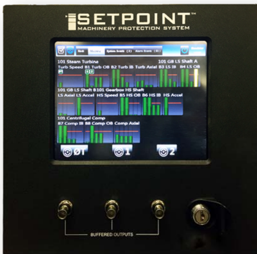
Figure 1: SETPOINT door and touchscreen showing its 3 programmable buffered output connectors
