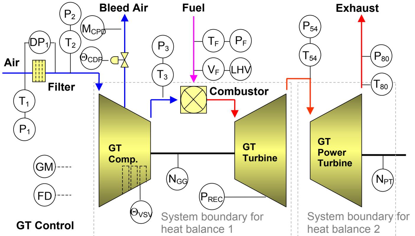
LM 2500 process measuring positions (these signals are easily imported to COMPASS™ and used for judging the performance condition of the gas turbine).
