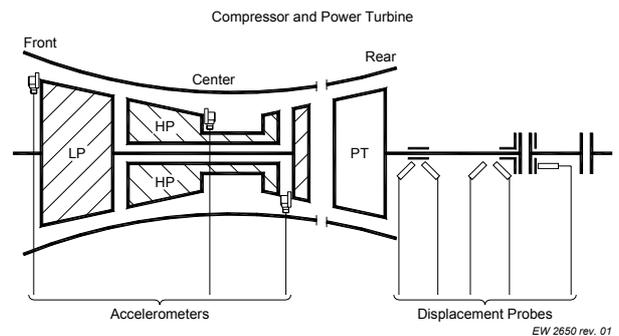
Vibration sensor instrumentation for a **Rolls-Royce RB211** gas turbine, comprising of a 2 shafts gas generator and a power turbine.
