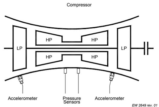
Vibration sensor instrumentation for a General Electric **LM 6000** gas turbine (2 shafts based on the twin spool principle).
