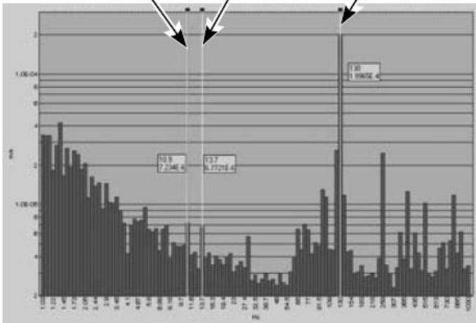
Before replacing speed regulator
