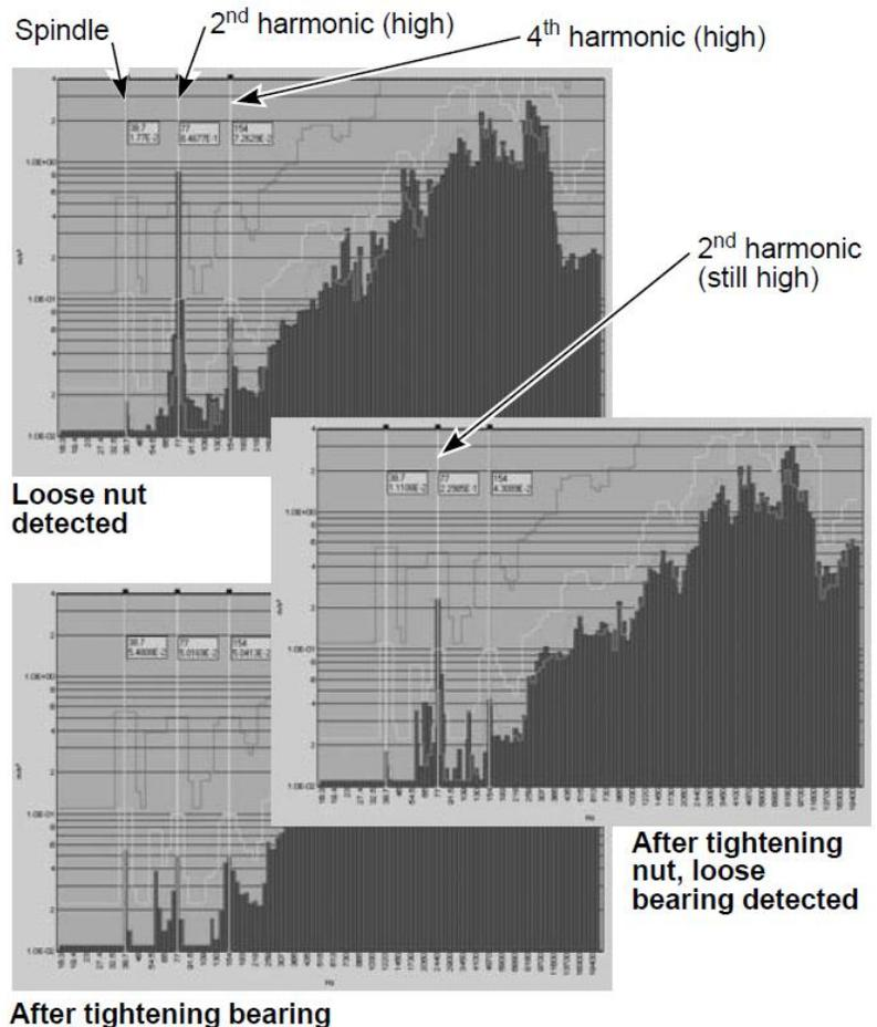
Figure 7. CPB plots showing mechanical looseness on multi-spindle lathe.
