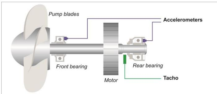
Figure 3. Sensor type and location for the Pentair Fairbanks Nijhuis propeller pump.
