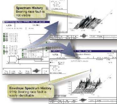
Figure 4. A developing fault in the cooling tower fan motor can be seen in the envelope spectrum plot above (it was not evident in the spectrum plot). The 91 Hz frequency indicates the fault was in the outer race, and further analysis revealed it was caused by brinnelling of the bearings.
