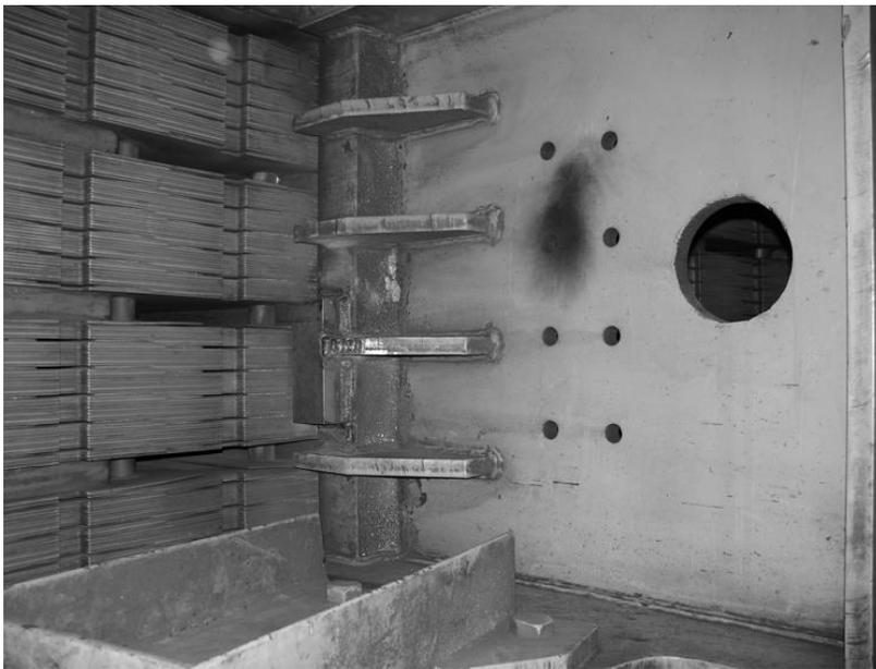
Figure 6. Modified rotor rim support structure.
