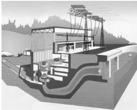
Figure 1. Żarnowiec pump storage hydroelectric power station. The 10.5 m diameter generators produce 179 MW from a 180 m<sup>3</sup>/s flow at 166.7 rpm.
