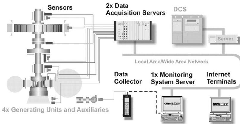
Figure 3. Monitoring system configuration (shown in colour).
