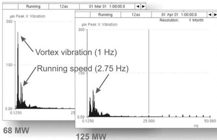
Figure 4. Detection and severity evaluation of the vortex rope turbulence using a spectrum plot. The example above shows the dominating presence of a frequency component indicative of a vortex (1/3x to 1/2x running speed) at 68 MW load (left). One month later at the same measurement point but at a higher load of 125 MW (right) there is little evidence of a vortex.
