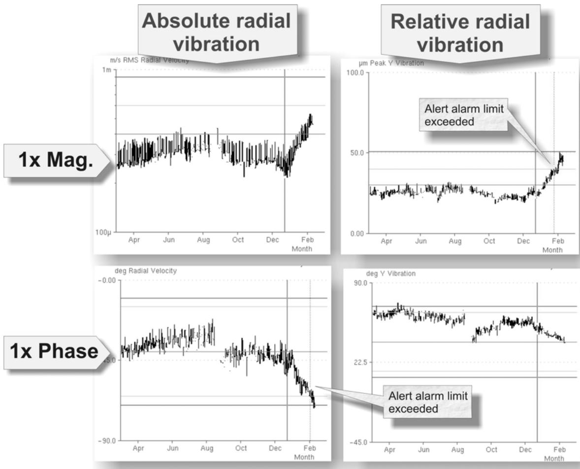
Figure 5. Vibration measurements from a radially-mounted accelerometer and displacement transducer on the unit 1 generator guide bearing showing a rapid change in magnitude and phase at around Christmas, 2002. As seen in the lower plots, accelerometers were more sensitive to phase change than the displacement transducers.
