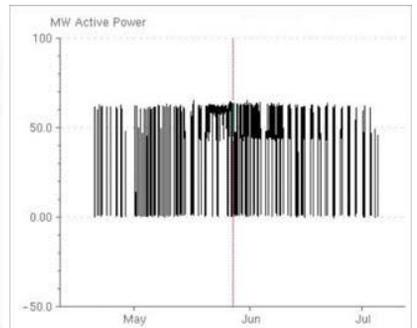
Figure 5. Active power plot showing the high number of starts and stops for unit 1 during a 2.5-month period. Part load operation can also be seen here.
