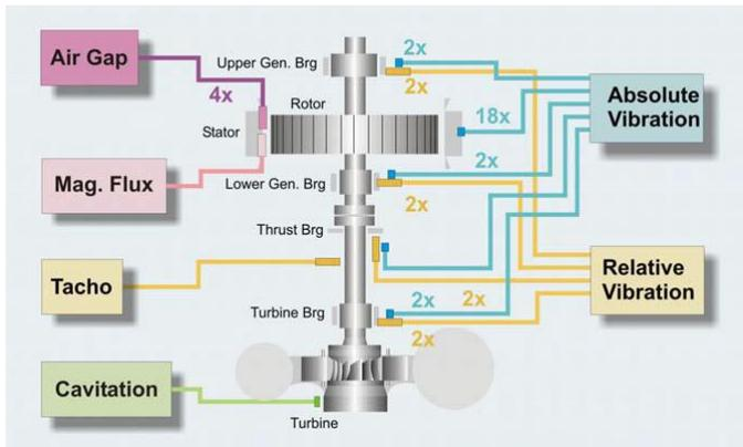
Figure 2. Sensors installed on the Momina Klisura generating units. Process parameters imported from the DCS are not shown here.
