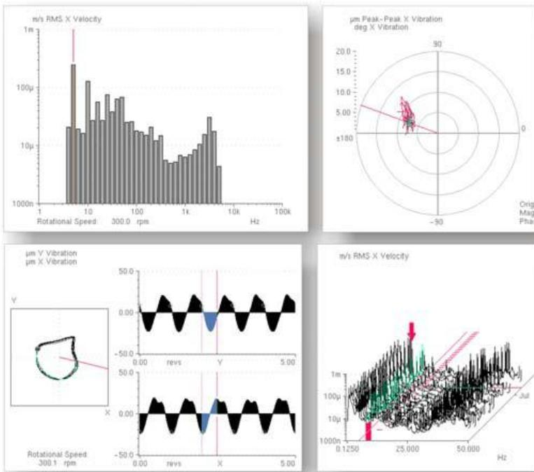
Figure 4. Example of plots for the upper generator bearing of unit 1. CPB spectrum at 23% bandwidth frequency (upper left), 2<sup>nd</sup> order vector history (upper right), orbit (lower left), and a waterfall FFT spectrum.
