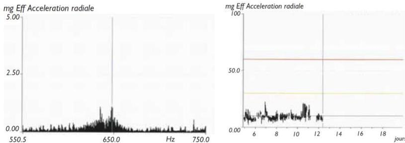
Figure 4. 5th octave chatter vibration from 4-stand mill shown in an FFT spectrum plot (left) and as a bandpass trend measurement (right).
