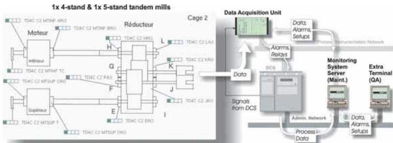
Figure 3. Condition monitoring system configuration for the 4 and 5-stand tandem mills at Tilleur.
