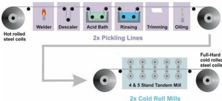
Figure 1. Tilleur has two pickling and two cold roll tandem mills.
