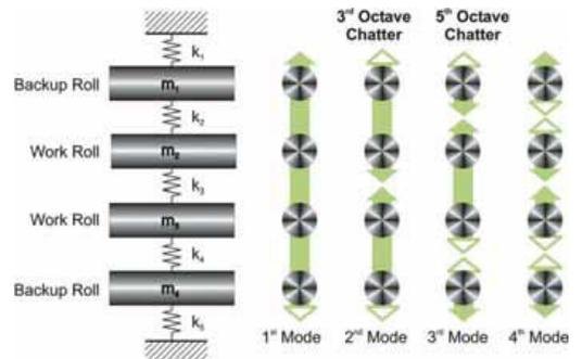
Figure 2. Vibration modes of a stand with four degrees of freedom.
