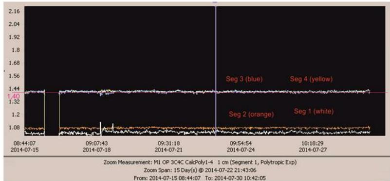
Figure 6. Cylinder 4 CE (stage 1) of a 2 stage, 2 cylinders per stage, double acting reciprocating compressor for gas compression (4 cylinders in total). The expansion line deviation is due to acoustic resonance of the dynamic pressure sensor, not due to a leaking valve.
