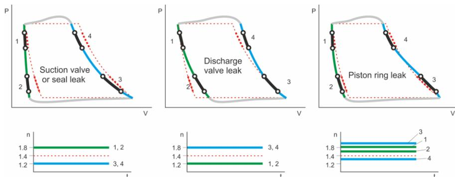
Figure 5. Examples of detecting cylinder leaks (shown in the PV plots), using the four calculated polytropic n values (shown below the PV plots). The theoretical PV plot is shown as a red dotted line, where n = 1.4 (based on the gas properties).
