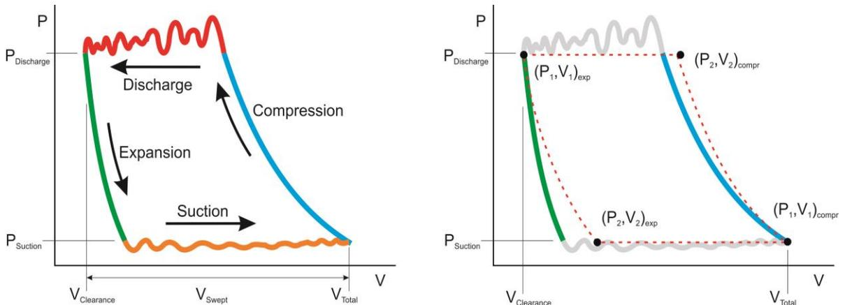
Figure 2. Left: PV plot showing the four basic compressor cycles. Right: Theoretical PV plot (red) overlying a PV plot. The deviation between the theoretical and actual expansion and compression curves indicate a suction valve leak in this example.
