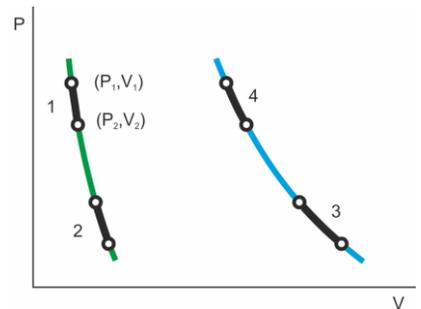
Figure 4. Example of locations for calculating n for four segments using Equation 2. The P and V values for segment 1 are indicated on the expansion line. (Green is the expansion line, blue is the compression line).
