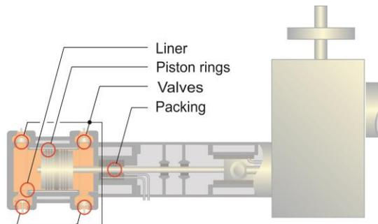
Figure 1. 2-cylinder reciprocating compressor shown, indicating where cylinder gas leaks can occur. The area in the cylinder where the compressed gas is located is shown in orange.
