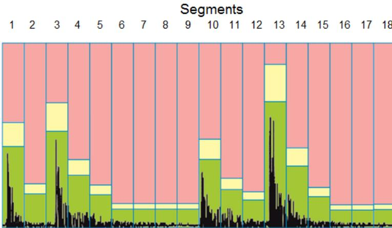
Figure 2. The individual events may be concentrated in a single segment or spread out over several. Each segment can be individual monitored to alarm limits (red is danger, yellow is alert and green is the reference). The segments shown above are equally spaced for one complete rotation of the crank. It is also possible to have segments with varying widths.
