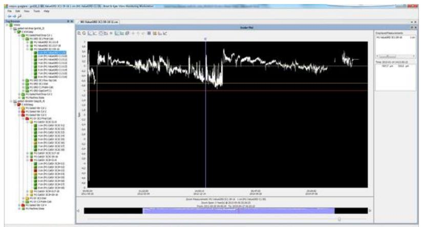
Figure 6. Long-term rod position signal from segment 9 of cylinder 1 of a 2-cylinder compressor.
