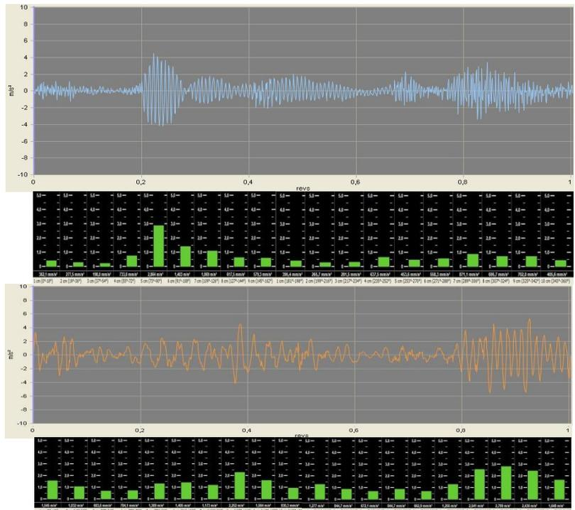
Figure 3. The vibration signal of the reciprocating compressor cylinder for one complete rotation of the crank. Top screen shows 20 RMS vibration bandpass segments at 18 degree crank position intervals for the cylinder head. Bottom screen shows the 20 segments for the crosshead vibration.
