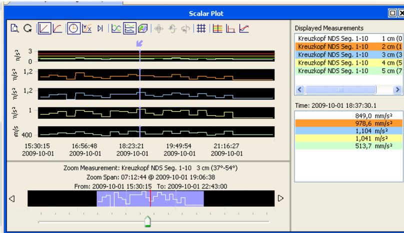
Figure 4. Gated vibration trend shown for the first 5 segments.
