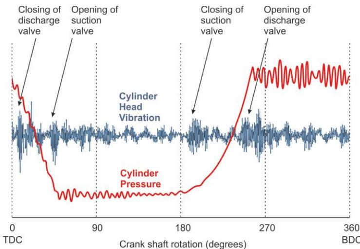
Figure 1. The cylinder head vibration time signal plotted against the cylinder pressure showing individual valve opening and closing events. Other vibration events not indicated here include pressure dynamics, pulsations within the cylinder and kinematics of the piston assembly movement.
