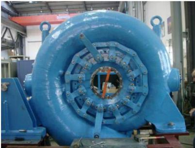
Figure 1. Andritz Hydro workshop in Schio, Italy. (The spiral case and distributor shown in the photo is actually part of several older units that are being reconditioned to be installed in rural South American towns through a non-profit organization. Retired Andritz Hydro factory workers are being asked to come back part time to do the reconditioning and commissioning.)
