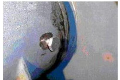
Figure 3. Typical accelerometer mounting for impact and frame vibration monitoring. Minimal downtime is required to install this.
