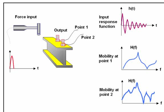
Fig. 1: The effect of different mobility on the spectrum appearance
