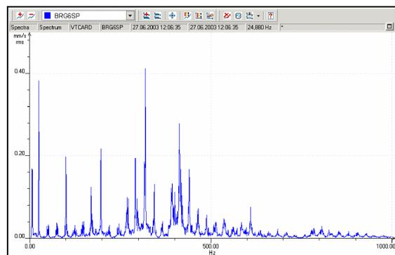
Fig. 3: Standard FFT spectrum showing apparent periodicity
