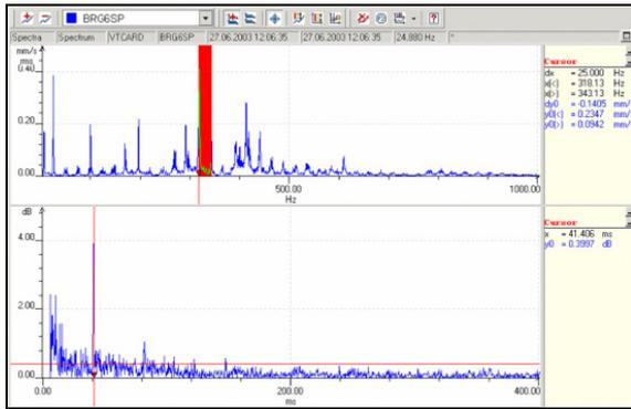
Fig. 4: The original FFT spectrum (top) and the corresponding Cepstrum (bottom)
