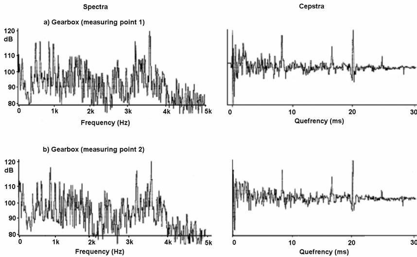
Fig. 2: Separation of source and transmission paths
