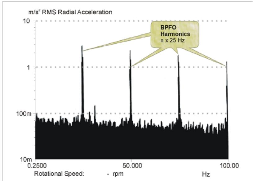
Figure 4. SED spectrum plot showing an outer-race bearing fault.
