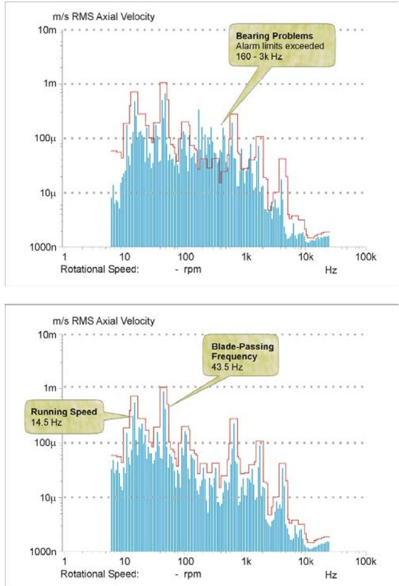
Figure 3. 6% CPB spectrum plots of a cooling fan at a gas processing plant. Lower plot shows a normal signature, upper plot shows resonances excited by a bearing fault.
