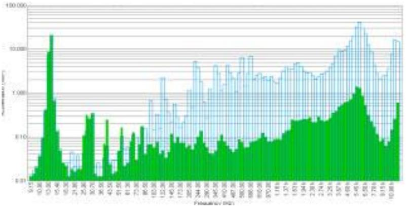
Figure 4. CPB6% plot showing increased medium and high frequency vibrations caused by excessive clearance in a rolling-element bearing (note that there is little change in the running speed frequency).
