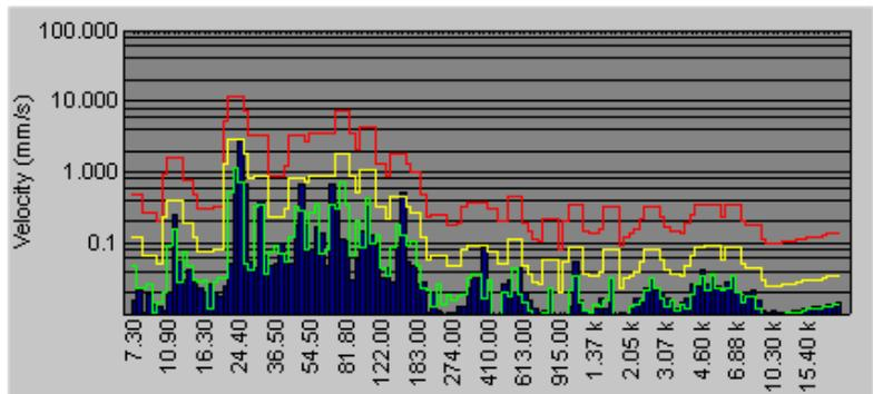
Figure 1. CPB23% spectrum measurement with alarm limits..
