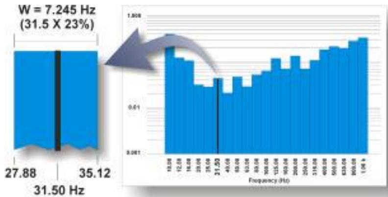
Figure 2. A CPB23% measurement from 10 to 1000 Hz has 21 frequency bars. In this example each bar has a bandwidth that is 23% of the center frequency.
