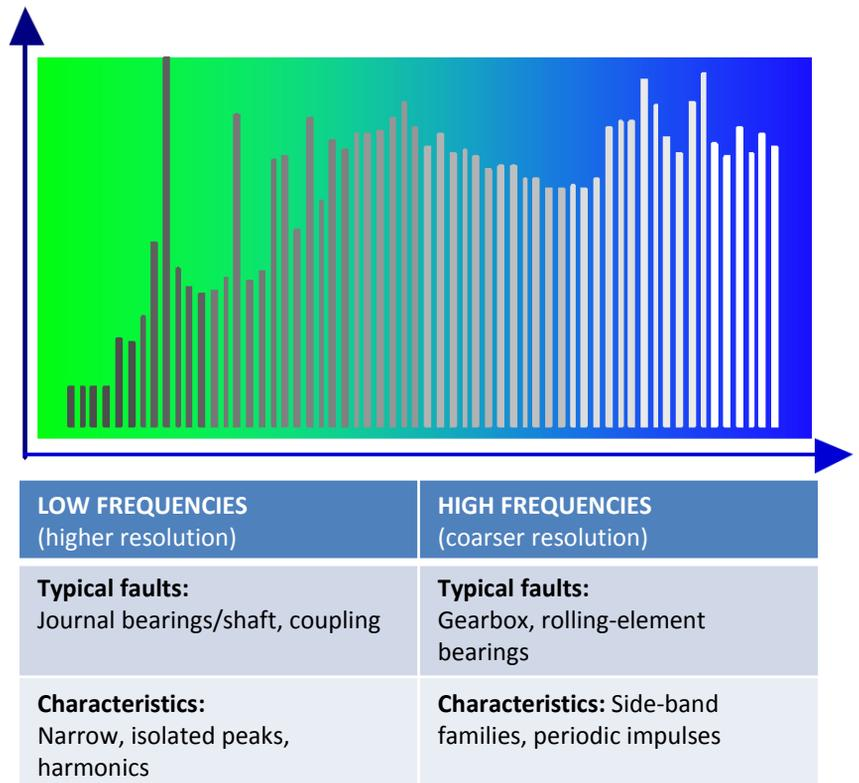
Figure 3. CPB has optimal resolution for detecting many kinds of faults.
