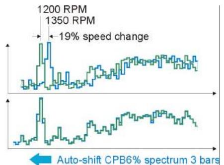
Figure 5. Example of an automatic speed compensation routine. In this example, each CPB bar is 6% wide, so a 19% speed change corresponds to moving the entire spectrum three lines.
