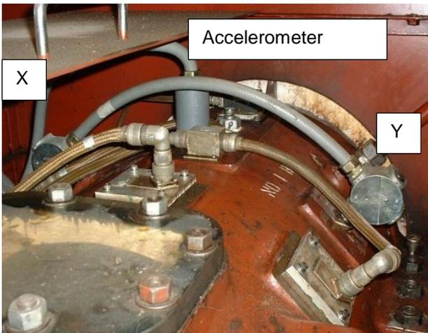
Figure 6 Bearing showing the X/Y transducers
