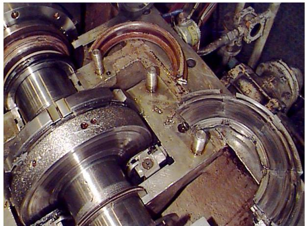
Figure 13 Feed pump thrust bearing failure
