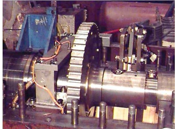
Figure 8 HP Differential expansion transducers
