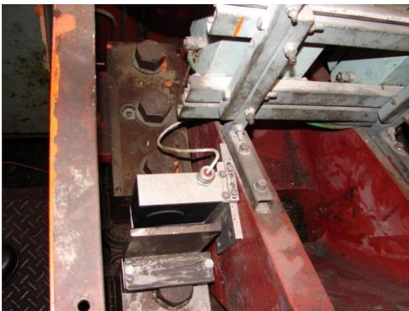
Figure 7 Casing expansion transducers
