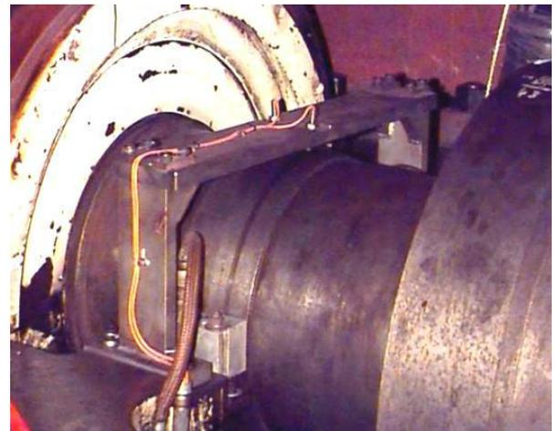
Figure 9 IP Differential expansion transducers
