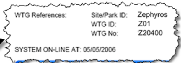
Heading showing turbine identification, and the time when the turbine went on-line.
