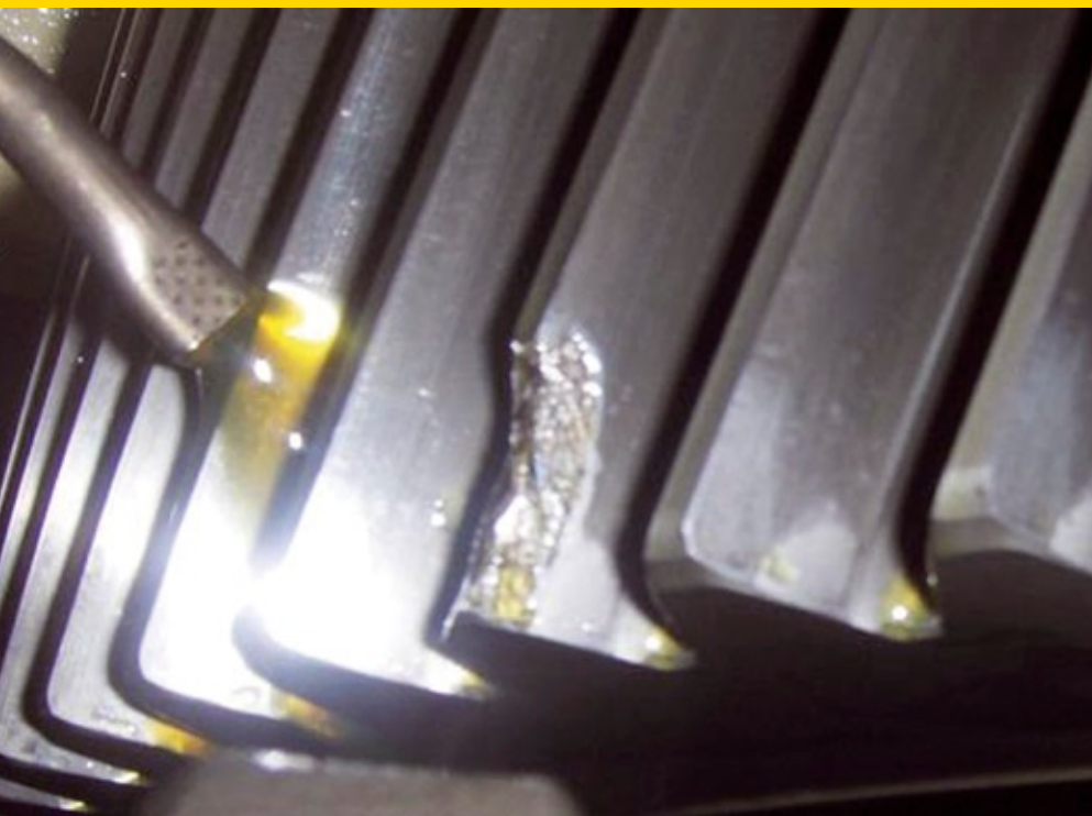
A chipped tooth on a wind turbine gearbox detected by our system.
