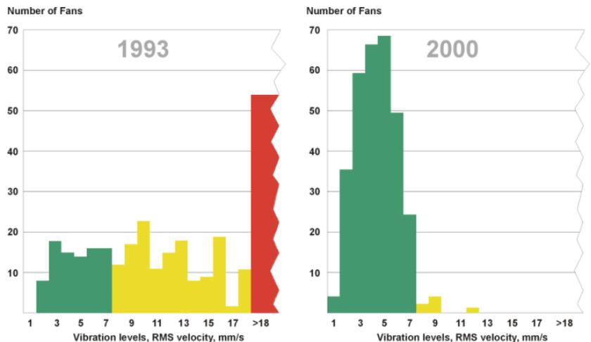
Figure 3. Offline monitoring has considerably reduced maintenance on the 897 fans. The number of fans operating within the allowable vibration levels (shown as green) according to ISO 2372 in 2000 has increased significantly since 1993.
