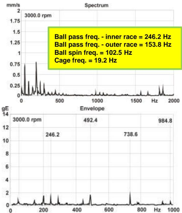
Figure 12. Before Repair (June 14): There is already evidence of damage to the inner ball bearing race as seen by the prominent ball passing frequency for the inner race (246.2 Hz) and its harmonics (492.4, 738.6 and 984.8 Hz).
