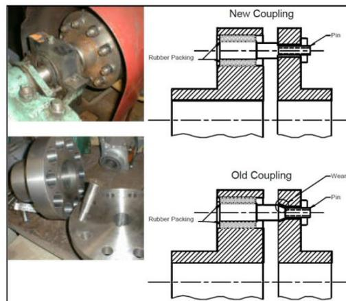
Figure 6. Flexible coupling of the accident confinement system pump showing newly designed pump-end flange and bolts.
