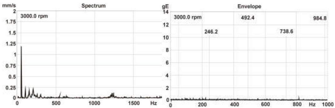
Figure 14. After Repair (July 20): The high frequency vibrations are reduced significantly in the spectrum plot, as are the peaks associated with the ball passing frequency for the inner race and its harmonics in the envelope plot.
