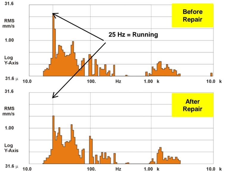
Figure 7. Constant percentage bandwidth spectrum (CPB) of the accident containment system pump before (above) and after (below) replacing the coupling with a new design.
