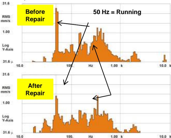
Figure 9. CPB spectrum of the purification and cooling system pump before (above) and after (below) replacing the impeller.
