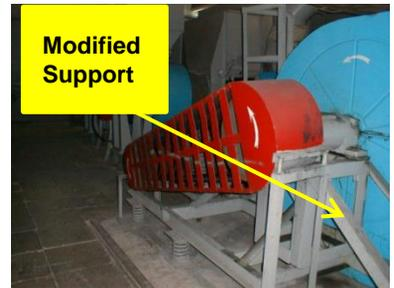
Figure 4. Horizontal belt-drive support modification for those fans that had excessive vibrations due to lack of structural stiffness.
