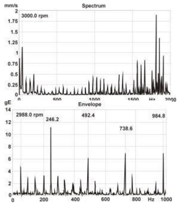
Figure 13. Before Repair (July 1): As the damage progresses, the spectrum plot shows increased vibration amplitude in the high frequency range. The ball passing frequency for the inner race and its harmonics are clearly seen in the envelope plot.
