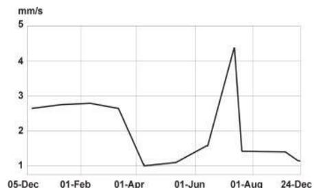
Figure 11. Vibration on the N4 bearing of the pump has increased from 1.6 mm/s June 14 to 4.3 mm/s July 14.
